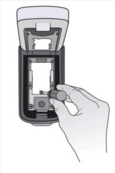
**4. Use a screwdriver to remove the screw from the code tamper plate.**
