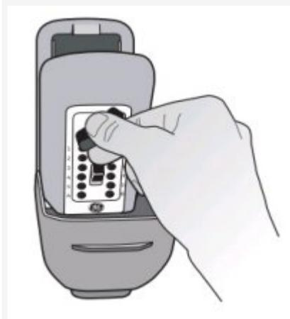
Turn the OPEN lever clockwise 180° to open. If the combination is set correctly, the OPEN lever will turn fully and the locking bolt will retract.
